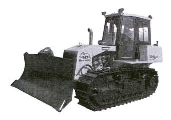
(b) **Dozer Model 'BD85':** Powered with 230 HP BEML turbocharged direct injection powerful diesel engine fitted with Power-shift transmission and Straight Tilt Dozer Blade
