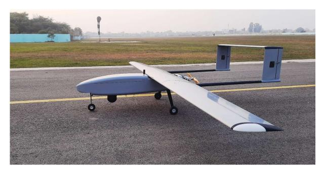
BEML is also displaying the 25 kg Class Tactical UAV being developed indigenously in collaboration with Indian Institute of Technology, Kanpur. The UAV is intended to carry versatile payloads of 3.0 kg, such as day & night cameras. It can take off and land in short runways, fly continuously for 8 hours and has 50 kms radio range.
